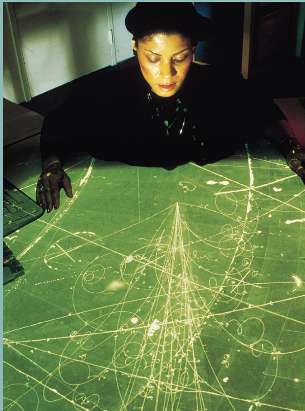
Figure 1. Curving lines in this “bubble chamber” photograph show the trajectories—and thus the identities—of various subatomic particles created by an accelerator. Careful measurement of these tracks (which Renee Jones of Fermi National Accelerator Laboratory is doing here for a 1984 experiment) reveals much about the undetected parent particles that give off such sprays. Like most practitioners now, the authors avoid this labor-intensive step by employing electronic detectors rather than bubble chambers in their current hunt for a special class of exotic particles, ones made (in whole or in part) of the very force that holds matter together.
